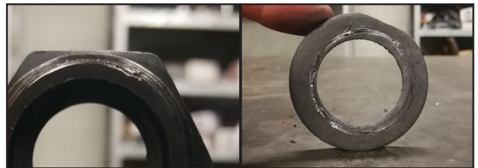
GALLING AT NUT-WASHER INTERFACE
